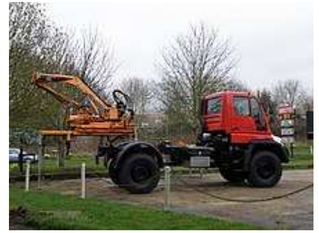
The modular design of the Unimog offers attachment capabilities for various different implements.
